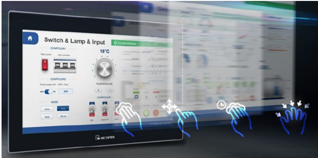
Figure 1: Maple Systems Capacitive HMI devices provide support for multi-touch gesture recognition. Touch gestures can trigger various actions such as change window, set bit, set word, execute macro, popup window, keyboard input, and screen hardcopy. Triggering a sequence of actions using a single gesture is also possible.
